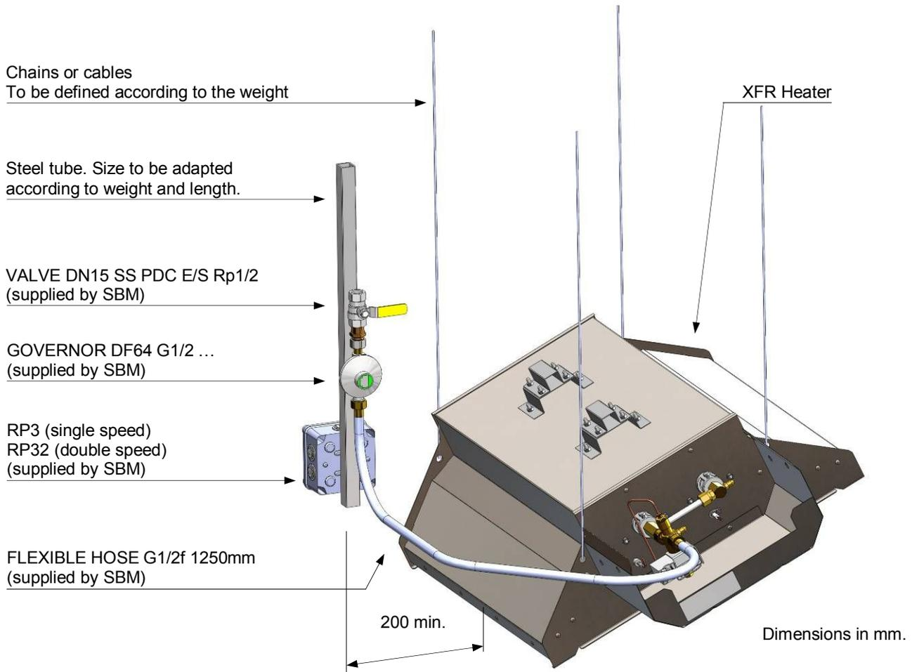
❑ Example of mounting bracket for **XFR 48-2** and **XFR 64-2**, to be supplied by the installer.
