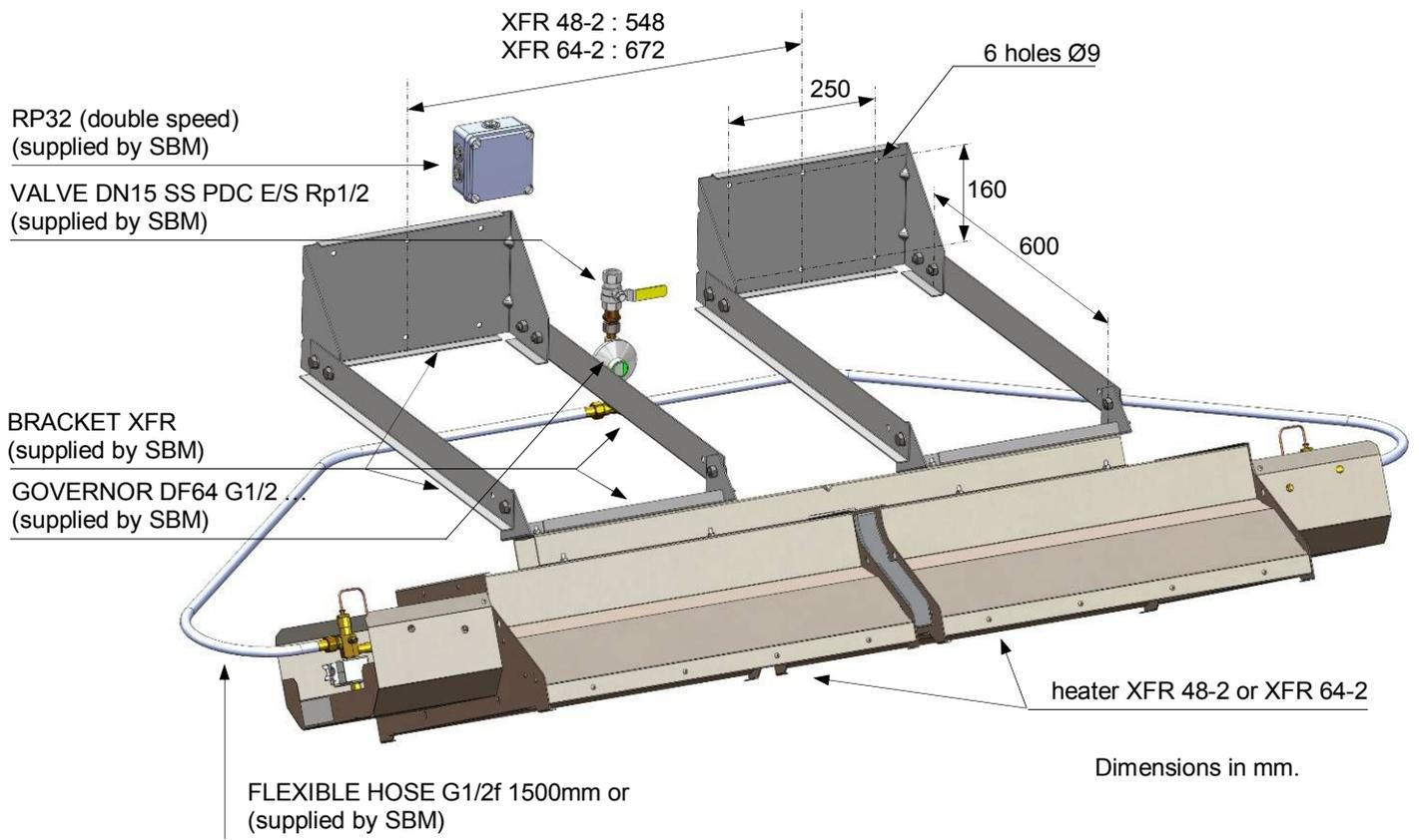
❑ Hanging exemple with chains or cables for **XFR 48-2** and **XFR 64-2**
